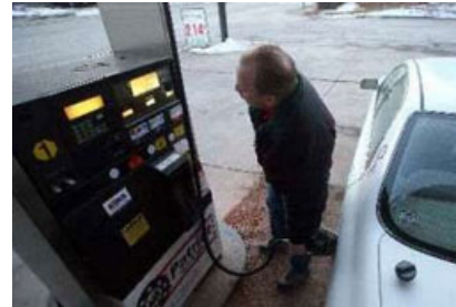
Mark Frederick fills up with E-20, a blend of 20 percent ethanol and 80 percent gasoline, at Canyon Lake Gas and Auto recently. The pump Frederick was using is a blender pump, which blends the ethanol and gas while pumping. Photo: Ryan Soderlin/Journal staff
